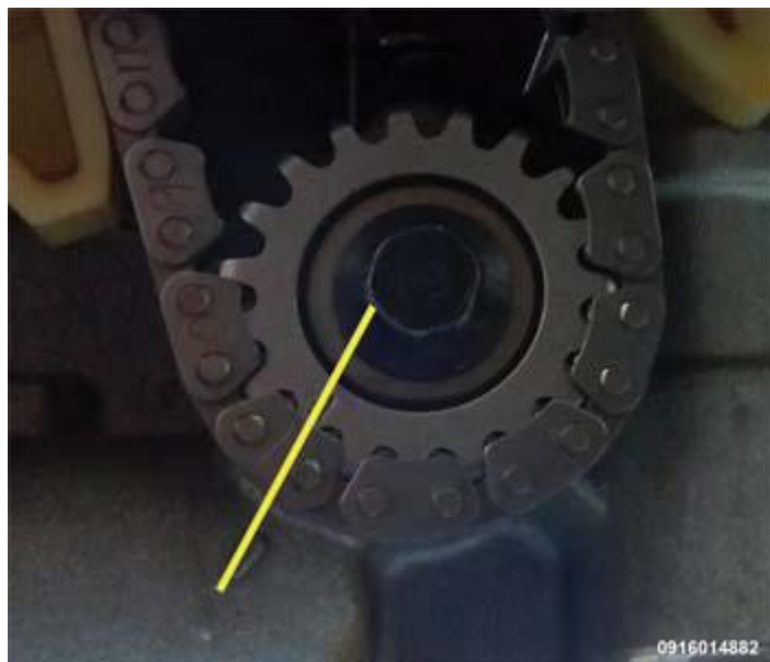
Fig. 340: Aligning Balance Shaft/Oil Pump Drive Gear And Housing Indicator Courtesy of CHRYSLER GROUP, LLC
