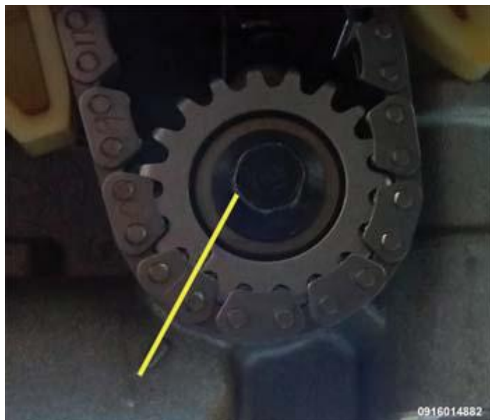
Fig. 345: Aligning Balance Shaft/Oil Pump Drive Gear And Housing Indicator Courtesy of CHRYSLER GROUP, LLC
