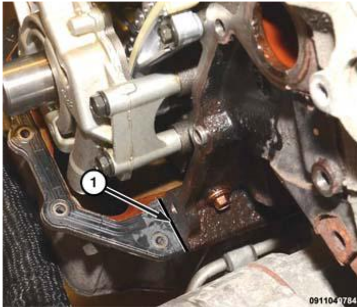
Fig. 422: RTV Sealant Application Area Courtesy of CHRYSLER GROUP, LLC
