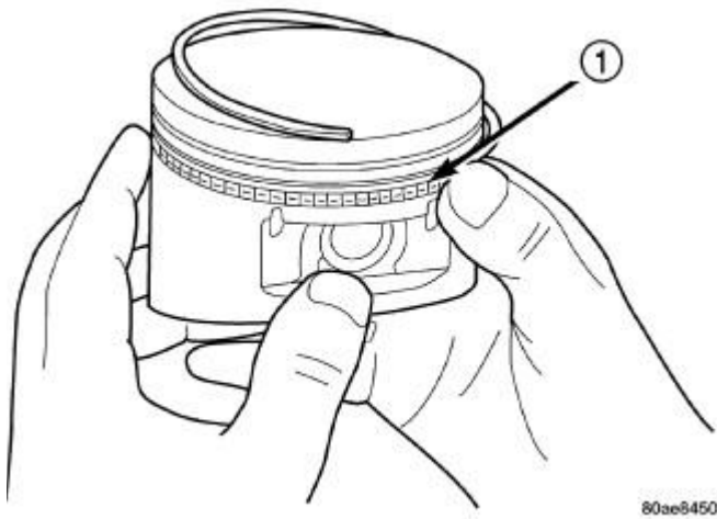
Fig. 221: Installing Piston Ring Side Rail Courtesy of CHRYSLER GROUP, LLC
