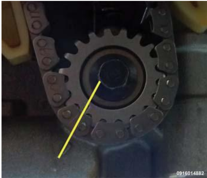
Fig. 301: Aligning Balance Shaft/Oil Pump Drive Gear And Housing Indicator Courtesy of CHRYSLER GROUP, LLC
