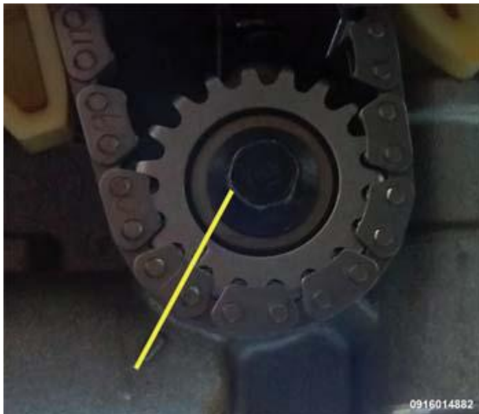
Fig. 296: Aligning Balance Shaft/Oil Pump Drive Gear And Housing Indicator Courtesy of CHRYSLER GROUP, LLC
