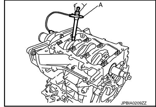
15. Install baffle plate.
