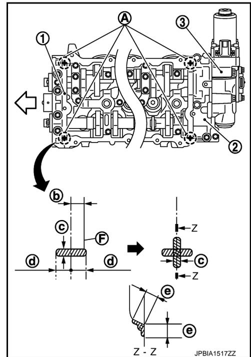
2. Install rocker cover gasket to rocker cover.
