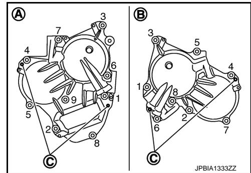
11. Install oil pan (lower). Refer to [EM-48, "Exploded View"](#).
