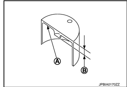
Available thickness of valve lifter (EXH): 27 sizes with range 7.88 to 8.40 mm (0.3102 to 0.3307 in) in steps of 0.02 mm (0.0008 in) (when manufactured at factory). Refer to [EM-144. "Camshaft"](#).
