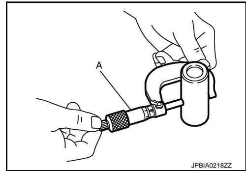
Connecting Rod Bushing Oil Clearance
