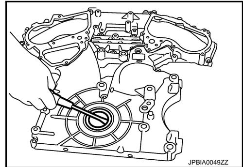
32. Remove O-ring (1) from rear timing chain case.
