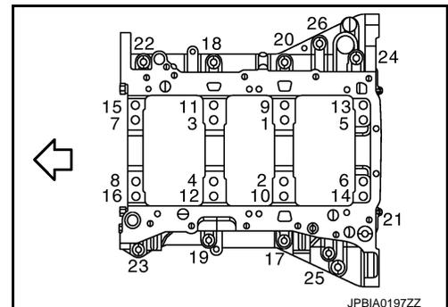
9. Remove lower cylinder block as follows:
