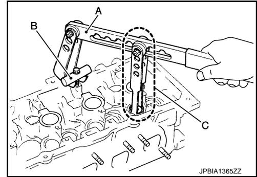
7. Remove valve spring retainer, valve spring and valve spring seat.
