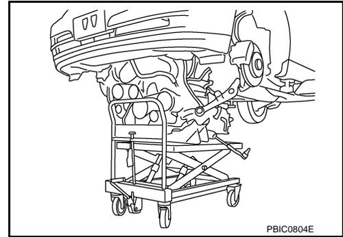
2. Remove rear engine mounting member bolts.
