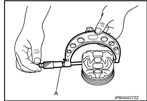
Piston-to-Cylinder Bore Clearance
