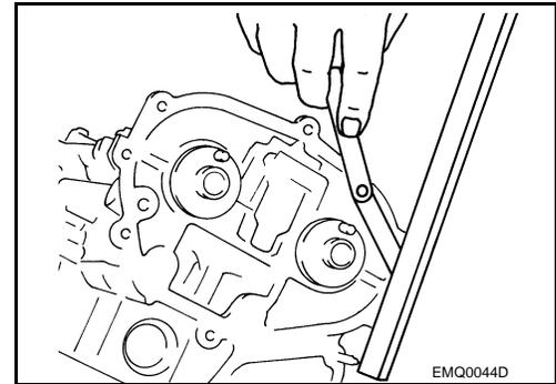
7. Install rear timing chain case. Refer to [EM-84, "Exploded View"](#).
