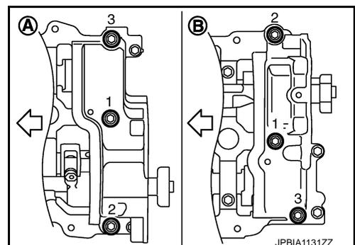
3. Remove front timing chain case, camshaft sprockets, and timing chain. Refer to [EM-54. "Exploded View"](#).
