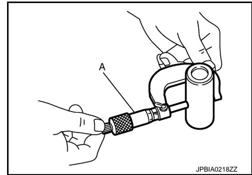
Piston to Piston Pin Oil Clearance
