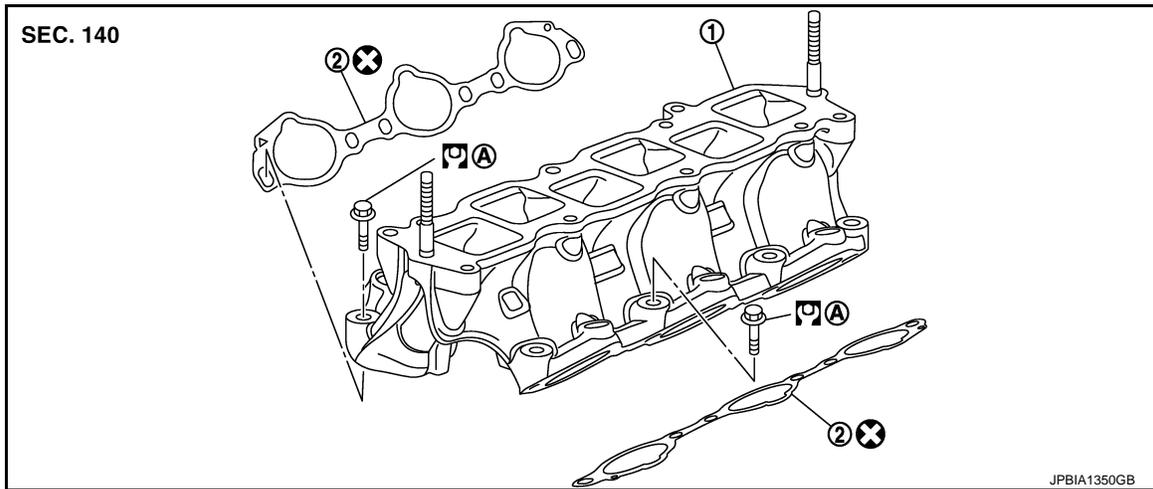
1. Intake manifold                      2. Gasket
