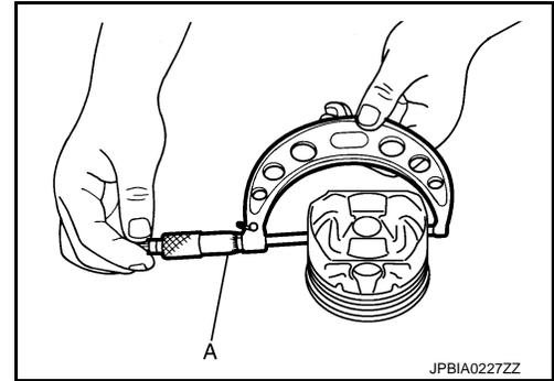
Piston-to-Cylinder Bore Clearance
