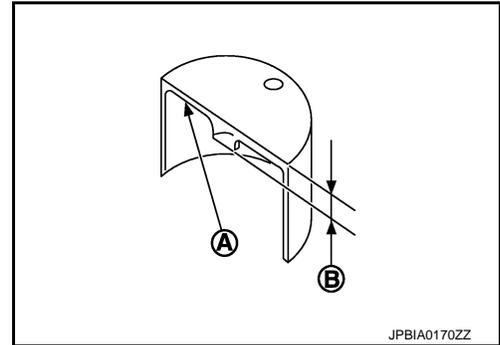
Available thickness of valve lifter (EXH): 27 sizes with range 7.88 to 8.40 mm (0.3102 to 0.3307 in) in steps of 0.02 mm (0.0008 in) (when manufactured at factory). Refer to [EM-145, "Camshaft"](#).
