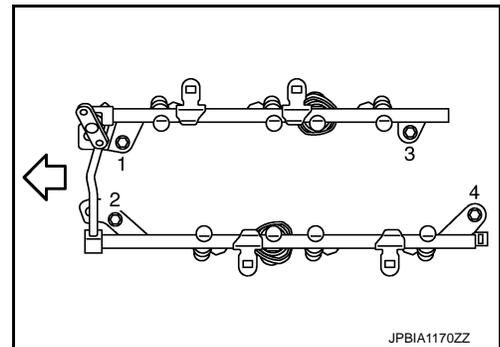
11. Remove fuel injector (2) from fuel tube (4) as follows:
