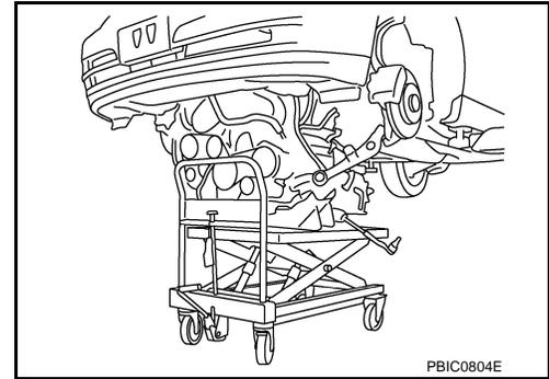
2. Remove rear engine mounting member bolts.
