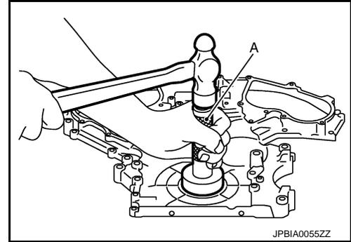
9. Install front timing chain case as follows:
