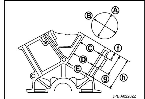
(Clearance) = (Cylinder bore inner diameter) – (Piston skirt diameter).
