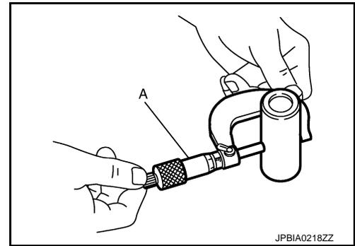
Connecting Rod Bushing Oil Clearance
