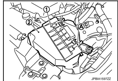
2. Remove holder (3) from air cleaner case (2), and then remove air cleaner filter (1) from holder.
