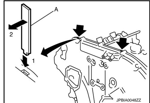
31. Remove front oil seal from front timing chain case using a suitable tool.
