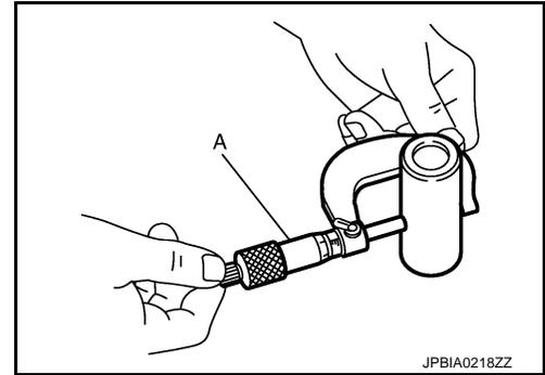
Piston to Piston Pin Oil Clearance
