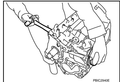
5. Remove connecting rod bearings from connecting rod and connecting rod bearing cap.
