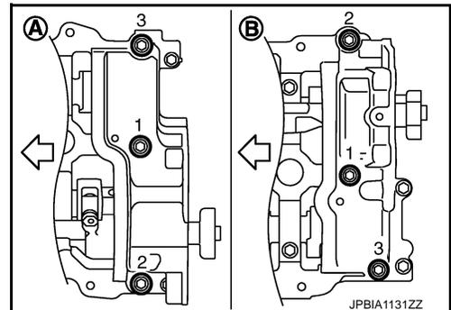
3. Remove front timing chain case, camshaft sprockets, and timing chain. Refer to [EM-55, "Exploded View"](#).
