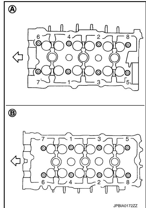
3. Remove cylinder head gaskets.
