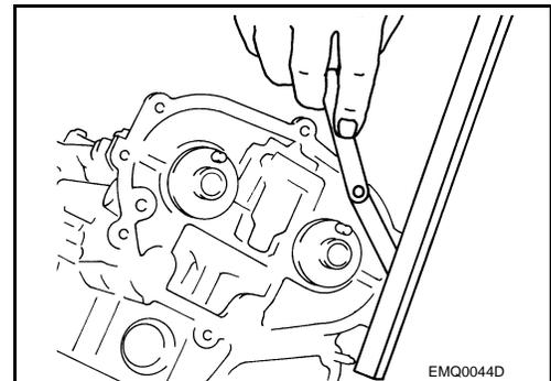
7. Install rear timing chain case. Refer to [EM-85, "Exploded View"](#).
