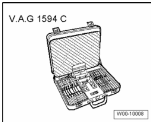
Fig. 157: Connector Test Set V.A.G 1594C
