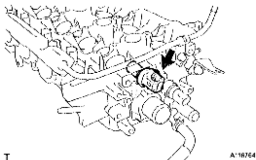
Fig. 157: Locating Camshaft Position Sensor And Bolt Courtesy of TOYOTA MOTOR SALES, U.S.A., INC.
