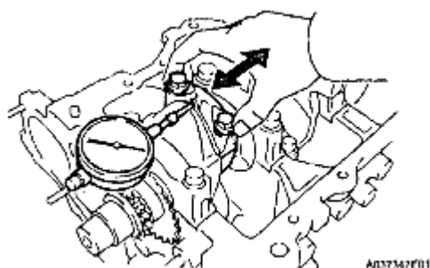
Fig. 419: Moving Connecting Rod Back And Forth Courtesy of TOYOTA MOTOR SALES, U.S.A., INC.
