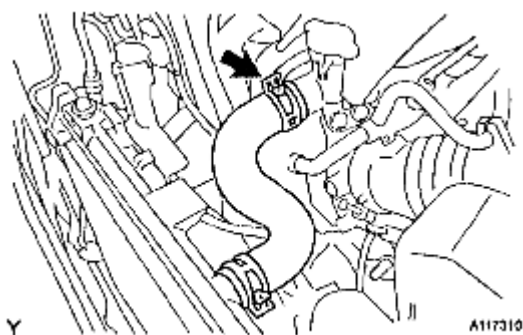
Fig. 268: Locating Radiator Hose From Water Filler Courtesy of TOYOTA MOTOR SALES, U.S.A., INC.
