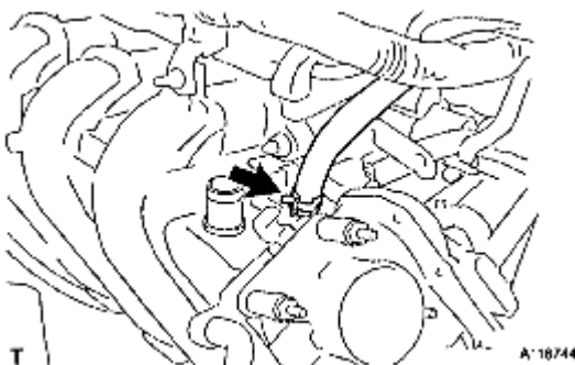
Fig. 234: Locating Union To Connector Tube Hose Courtesy of TOYOTA MOTOR SALES, U.S.A., INC.
