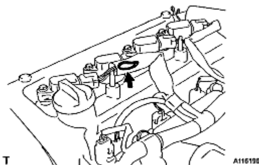
Fig. 1: Locating Wrap Wire Harness With Tape Courtesy of TOYOTA MOTOR SALES, U.S.A., INC.
