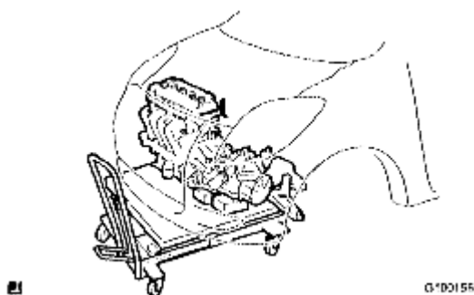
Fig. 321: Identifying Engine Lifter
