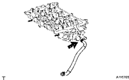
Fig. 207: Locating Water Bypass Hose Courtesy of TOYOTA MOTOR SALES, U.S.A., INC.
