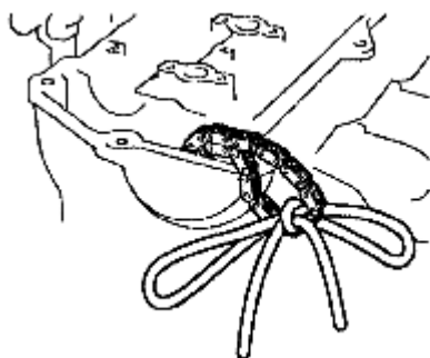
Fig. 91: Identifying Tie Chain With Piece Of String
