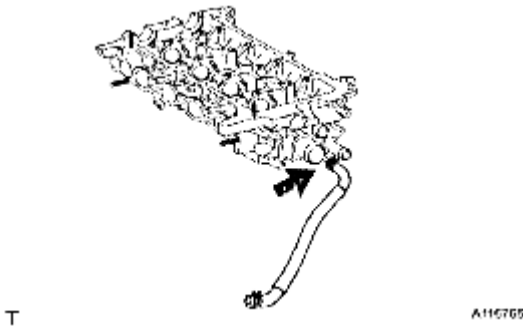
Fig. 159: Locating Water Bypass Hose Courtesy of TOYOTA MOTOR SALES, U.S.A., INC.
