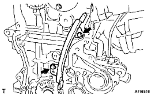
Fig. 66: Identifying Chain Vibration Damper With Bolts Courtesy of TOYOTA MOTOR SALES, U.S.A., INC.
