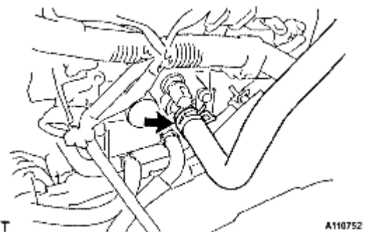
Fig. 145: Locating Heater Water Inlet Hose Courtesy of TOYOTA MOTOR SALES, U.S.A., INC.
