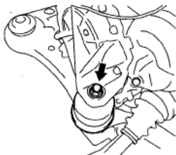
Fig. 136: Locating Nuts And Engine Mounting Insulators RH And LH Courtesy of TOYOTA MOTOR SALES, U.S.A., INC.
