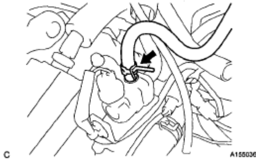
Fig. 162: Locating No. 1 Fuel Vapor Feed Hose Clamp Courtesy of TOYOTA MOTOR SALES, U.S.A., INC.
