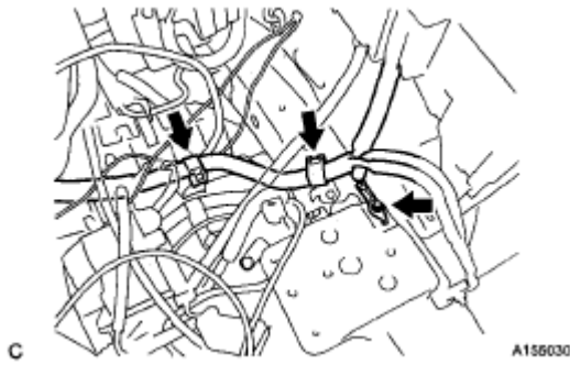
Fig. 146: Locating Bolt And Clamps On Body Courtesy of TOYOTA MOTOR SALES, U.S.A., INC.
