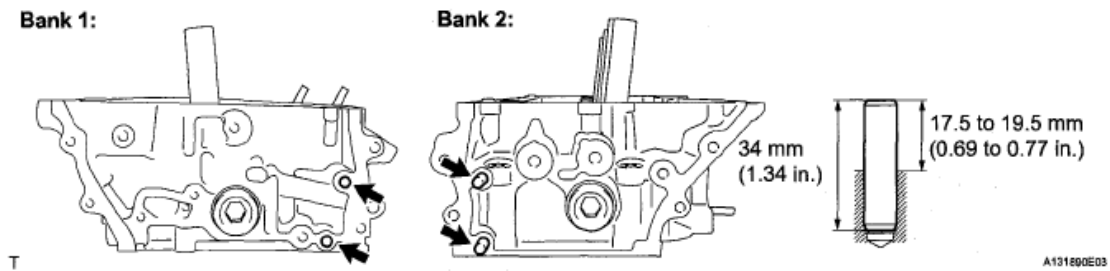
Fig. 403: Identifying Straight Pin Installation Procedure Courtesy of TOYOTA MOTOR SALES, U.S.A., INC.
