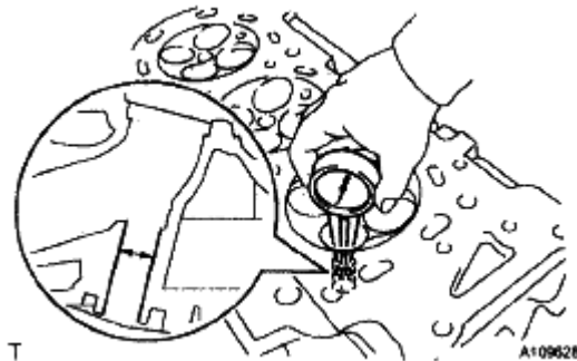
Fig. 396: Checking Bush Bore Diameter Of Cylinder Head
