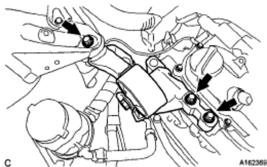
Fig. 163: Locating Bolts On Engine Moving Control Rod Courtesy of TOYOTA MOTOR SALES, U.S.A., INC.
