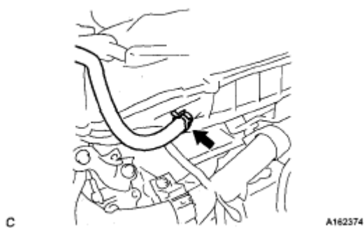
Fig. 161: Locating Union To Check Valve Hose Clip Courtesy of TOYOTA MOTOR SALES, U.S.A., INC.
