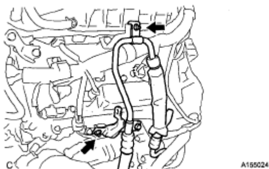
Fig. 74: Locating Power Steering Oil Pressure Switch Connector Courtesy of TOYOTA MOTOR SALES, U.S.A., INC.
