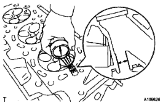
Fig. 393: Checking Bush Bore Diameter Of Cylinder Head Courtesy of TOYOTA MOTOR SALES, U.S.A., INC.
