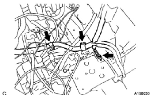
Fig. 69: Locating Bolt And Clamps On Body Courtesy of TOYOTA MOTOR SALES, U.S.A., INC.
