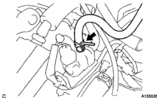
Fig. 54: Locating No. 1 Fuel Vapor Feed Hose Clamp Courtesy of TOYOTA MOTOR SALES, U.S.A., INC.
