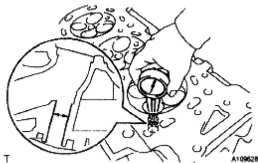
Fig. 396: Checking Bush Bore Diameter Of Cylinder Head
