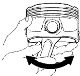
Fig. 280: Checking Fitting Condition Between Piston And Piston Pin Courtesy of TOYOTA MOTOR SALES, U.S.A., INC.
