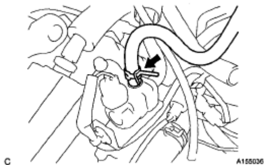
Fig. 162: Locating No. 1 Fuel Vapor Feed Hose Clamp Courtesy of TOYOTA MOTOR SALES, U.S.A., INC.
