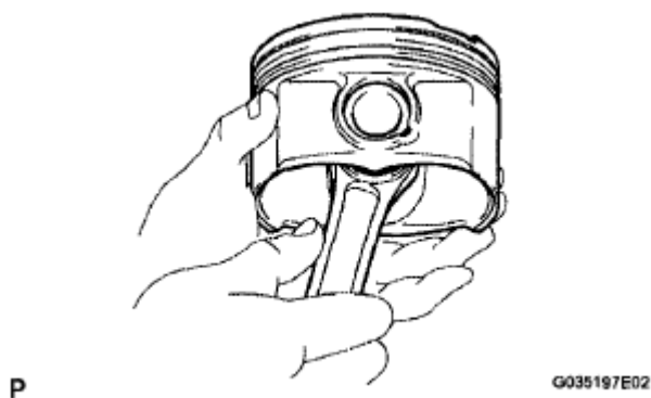
Fig. 394: Checking Fitting Condition Between Piston And Piston Pin Courtesy of ABLE BODY CORP.
